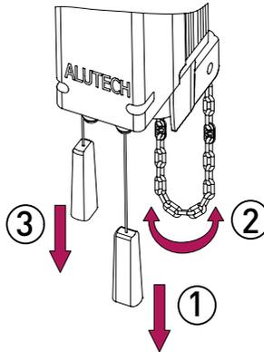
Figure 5. Emergency manual control using chain operation
