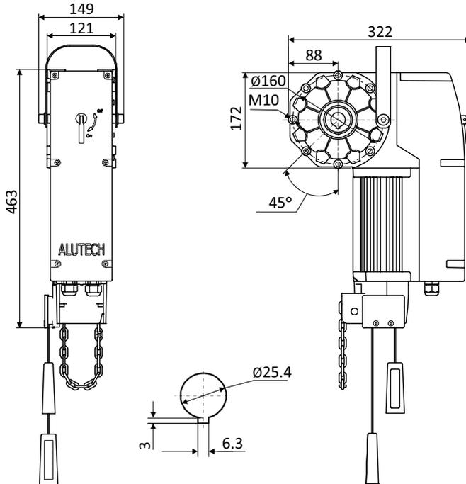
Figure 2. Dimensions of TR-10024-400 and TR-13018-400 drives
