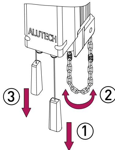
Figure 4. Emergency manual control using chain operation
